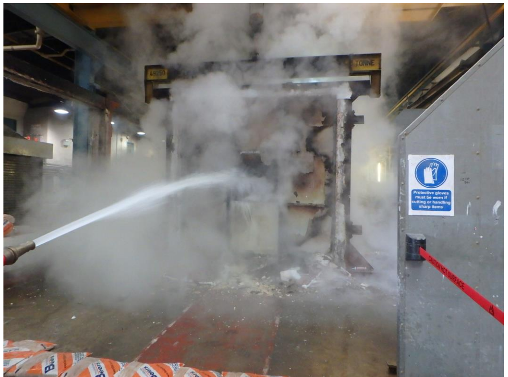
The exposed face of the assembly during the hose stream test
