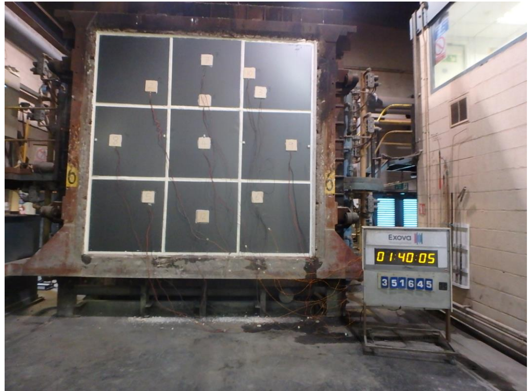
The unexposed face of the assembly after 100 minutes of testing
